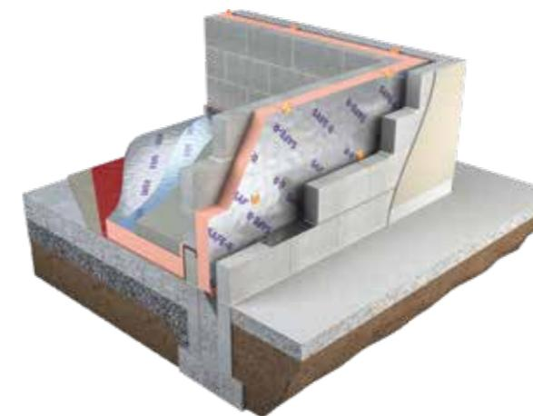
SR019/CW partial fill cavity wall insulation is the solution of choice to achieve the lower U-Values asked for under the building regulations whilst maintaining a residual cavity as a protection from wind driven rain.
